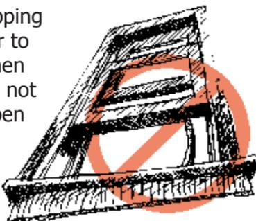
**SOLUTION:** Repair counterweight system or install hardware so the window will stay open securely or replace window.
