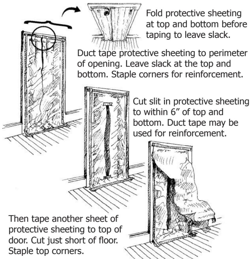
**In addition to the steps outlined in the section on setting up the work area, high dust jobs require containment of doors that allow access but prevent the migration of dust.**
