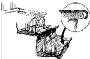
**SOLUTION:** Install a tight-fitting nose tread, or install a staircase runner.
