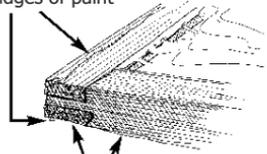
Seal this bottom edge very well, particularly the end grain. Use linseed oil or other sealant
