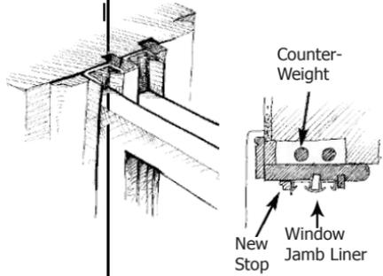
Cut flange of jamb liner with Plexiglas cutter.
